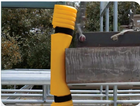
Rack Mounted Guard exceeded impact requirements of EN 15512.
